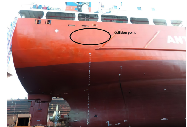
Hole in hull approximately five metres long. (Source: Anthony Veder)
