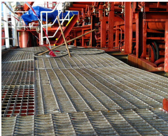
Displaced deck and manifold after the tank explosion
