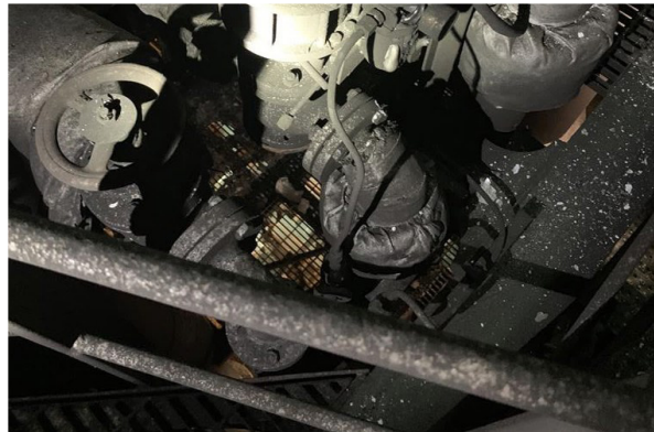
Damage after fire on board Curacao Trader. (Source: Crew)
