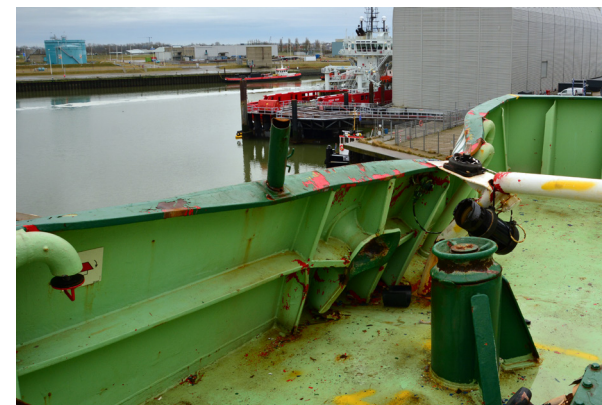
Damage to the stern after the collision
