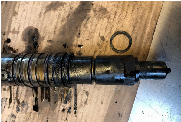
Damage to the injector bush of the main engine of the Peak Bilbao. (Source: Crew of the Peak Bilbao)
