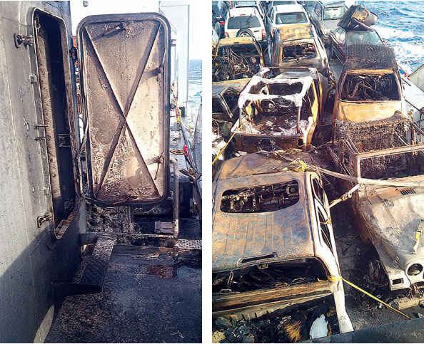
Left: Access door to the fore part of the Beauforte. Right: Fire damage to the cargo of the Beauforte. (Source pictures: Vertom Bereedungs gmbh)
