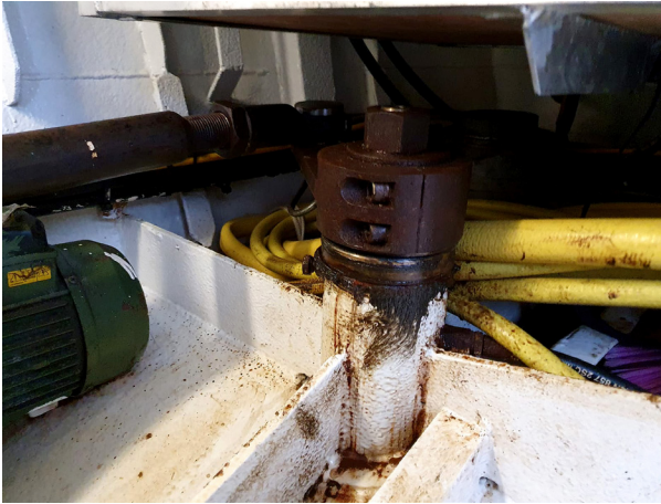
Securing mechanism of the rudder stock on the Libertas. (Source: Braveheart Maritiem)
