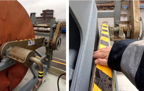
Left: Hose reel on board the Kroonborg. Right: Position where the crew member injured his hand on board the Kroonborg. (Source pictures: Wagenborg)
