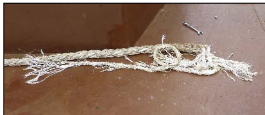
Figure 8: Photo of the port mooring line fracture surface
