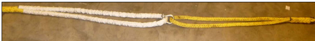
Figure 4: Example of a comparable mooring line extension as used during the mooring manoeuvre
