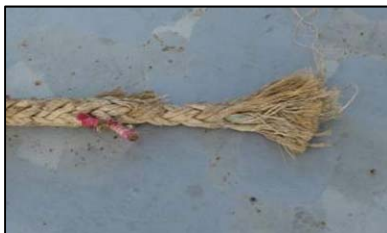
Figure 7: Photo of the starboard mooring line fracture surface
