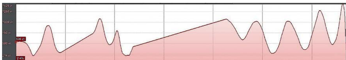
Figure 4: Altitude profile during the activation of the EGPWS over the North Sea.
