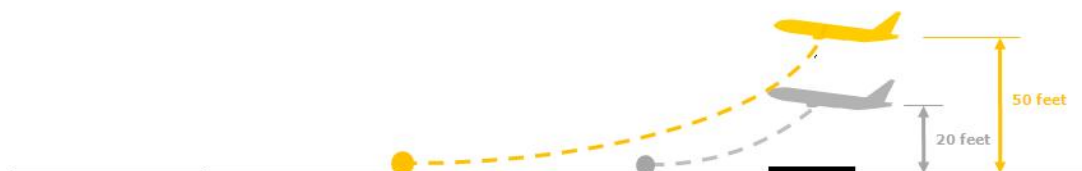
Figure 4: schematic reproduction of the flare manoeuvre at 20 feet (grey) and the flare manoeuvre at 50 feet (yellow) of the event flight with the touchdown points on the runway
