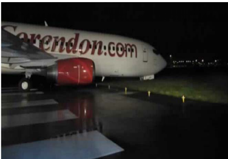
Figure 1: TC-TJF after overrunning Runway 22 with its nose off the paved surface (Source: Amsterdam Airport Schiphol)
